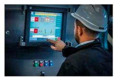
GHT F filter presses are provided with a PLC-based automation system complete with a human-machine interface (HMI) which simplifies monitoring of the filter operation and diagnosis of faults. Additionally, it allows for continuous adjustment of filtration parameters in order to optimize the variable requirements of the process.
