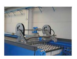
The automatic in-situ cloth washing system, which is programmable according to the user's needs, uses high pressure wash water and directional sprays to effectively regenerate the filter cloth permeability. The results are filter cloths with more consistent filtration performance and longer life.
