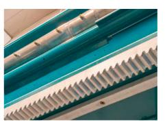
The automatic plate-shaking device, which is programmed to occur after the plate pack fully opens, ensures the filter cakes are properly discharged and removes possible cake fragments from the cloths. This system, along with the cloth rinsing system, allows the filter to run automatically and without operator assistance.
