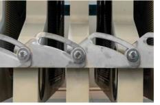
The cake discharge time is significantly reduced compared to traditional plate opening-closing systems with the use of an accordion-style plate pack opening and closing system. This fast operation increases the filter's throughput production.
