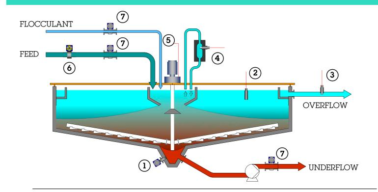
Control philosophy and instrumentation can be optionally provided for different levels of control responding to the client's needs. Typical controls involve flocculant consumption, overflow clarity and consistent underflow density.
